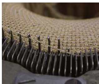
FIGURE 39 Circular knit machine Garments are shaped by varying yarn tension and stitch height during knitting.
